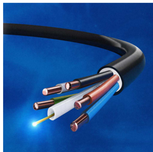
Fig. 1. 1 kV service cable with tube for blown fibre
